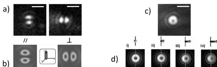
**Figure 1:** a) & c) Measured PSFs of single emitters strongly oriented along Z axis with, a), and without, c), polarization splitting. b) & d) Corresponding theoretical simulations of PSFs, reproduced from [2], b), and [3], c).
