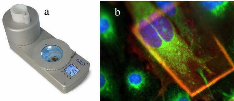
Cryo-fluorescence stage Linkam CMS196 (a) and cryo-widefield fluorescence of mouse embryonic fibroblast cells on quantifoil gold finder grids, imaged during the 2015 cryo-workshop at the Crick Institute, London.
