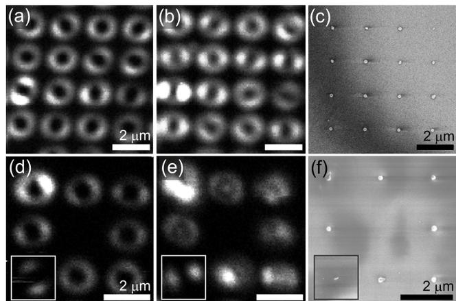
**Figure 1:** SHG images of an array of (a,b) gold nanobumps and (d,e) gold nanocones using focused azimuthal (a,d) and radial polarizations (b,e). Representative top-view scanning electron microscopy (SEM) images of (c) gold nanobumps from the same array and (f) corresponding gold nanocones. Insets (d-f) correspond to SHG and SEM images of a gold nanorod on the same substrate.
